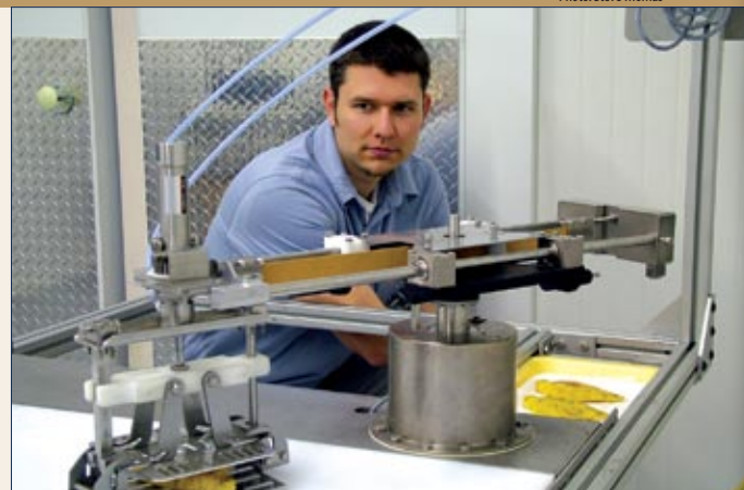
Researcher engineer Jonathan Holmes watches the operation of a washable robot designed for use in the food processing industry.
