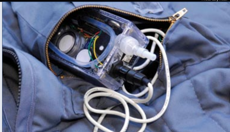
A sensor system worn in the pockets of a vest may help pinpoint triggers for asthma attacks.
