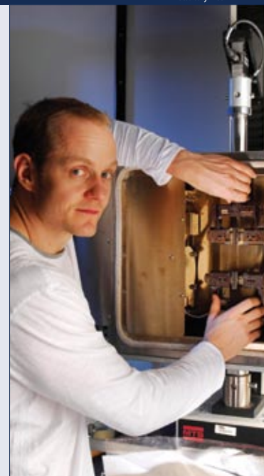
Professor Ken Gall reaches inside a test frame used to study shape-memory polymers.
