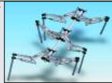
ABOVE: The Compact Rescue Crawler robot will have six legs — creating a bug-like appearance — to increase its maneuverability.
