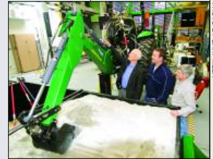
ABOVE: Professor Wayne Book and his robotics research team have developed a haptic backhoe system that gives the operator the sense of touching a wall when approaching a utility line.
