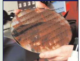
ABOVE : Professor John Cressler is reflected in a 200 GHz silicon-germanium integrated circuit wafer.
