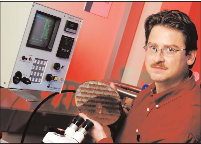
ABOVE: Professor John Cressler holds a 200 GHz silicon-germanium integrated circuit wafer at a cryogenic probe station capable of measuring temperatures to 200 degrees below zero Celsius.
