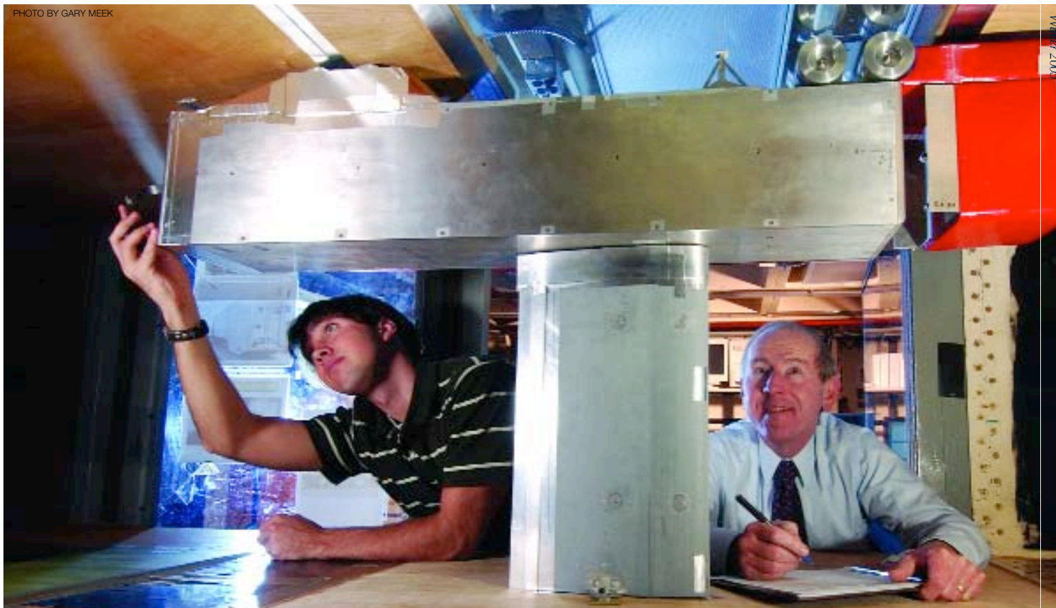
Researcher Robert Englar (right) and co-op student Daniel Hegeman adjust blowing slots on a model truck inverted in GTRI's low-speed wind tunnel. The testing helped assess the value of fuel-saving improvements.
