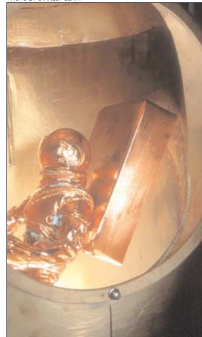
A scale model of an astronaut wearing a Russian-designed spacesuit was used to study antenna patterns inside the crew air lock designed for the International Space Station. The model was coated with copper to simulate the conducting layer in the spacesuit.
