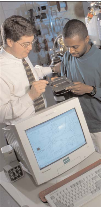
Gary Gray (left) and Comas Haynes analyze fuel cell components under development in the Georgia Tech Research Institute. Behind them is a reformer that produces hydrogen from natural gas.
