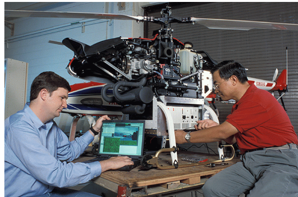
Eric Johnson (l) and Jeong Hur adjust controls of the GTMAX test bed UAV helicopter.
