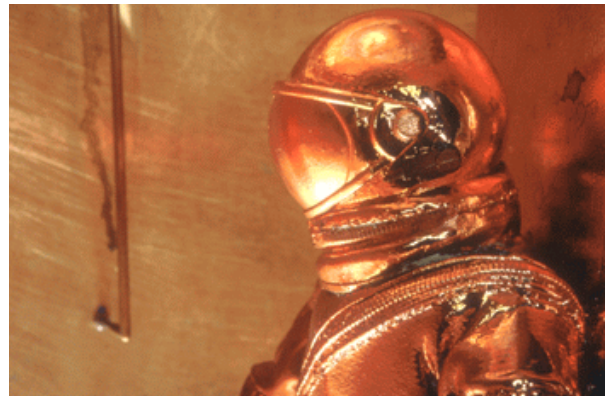
Georgia Tech researchers used this scale model astronaut inside a scale model crew air lock to design a special antenna needed to maintain communication with the International Space Station's crew.
