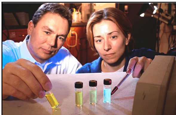
Researchers Marcus Weck and Amy Meyers examine vials containing dilute solutions of polymers with functionalized Alq3. By allowing the fluorescent material to be applied as a polymer, the researchers could help lower the cost of manufacturing organic light-emitting diodes.
