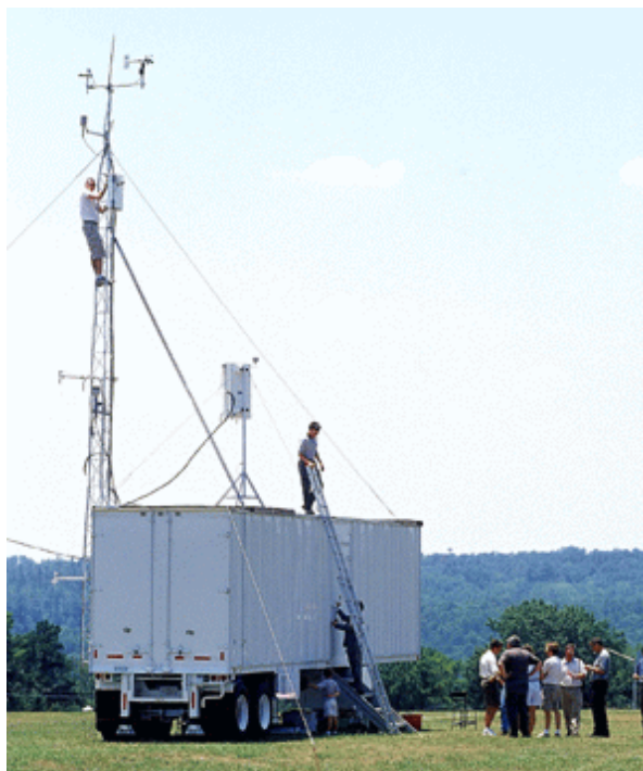
Atmospheric scientists at Georgia Tech are studying ozone levels in three Georgia cities: Augusta, Columbus and Macon. They use a mobile air quality monitoring unit to gather measurements.
